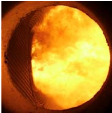
Figure 4 Flame from NR3 burner at Minimum Load (Type B Coal)
